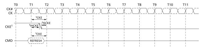
Note: 1. CKE can go LOW <sup>t</sup>IHCKE after the clock on which the REFRESH command is registered.
