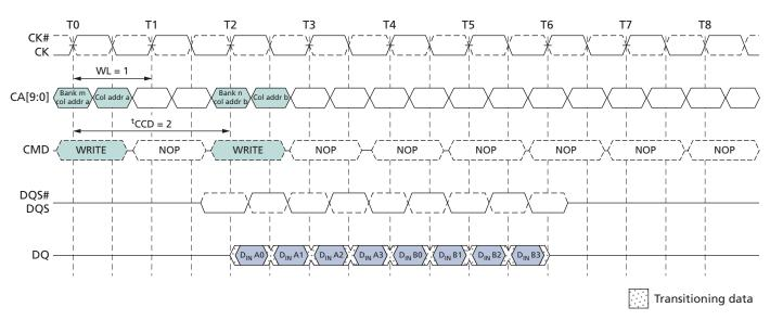
Note: 1. The seamless burst WRITE operation is supported by enabling a WRITE command every other clock for BL = 4 operation, every four clocks for BL = 8 operation, or every eight clocks for BL = 16 operation. This operation is supported for any activated bank.
