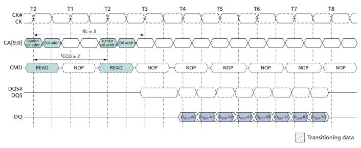
A seamless burst READ operation is supported by enabling a READ command at every other clock cycle for BL = 4 operation, every fourth clock cycle for BL = 8 operation, and
