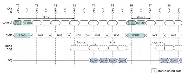
The minimum time from the burst READ command to the burst WRITE command is defined by the read latency (RL) and the burst length (BL). Minimum READ-to-WRITE latency is RL + RU( $^t$ DQSCK(MAX)/ $^t$ CK) + BL/2 + 1 - WL clock cycles. Note that if a READ burst is truncated with a burst TERMINATE (BST) command, the effective burst length of the truncated READ burst should be used for BL when calculating the minimum READ-to-WRITE delay.
