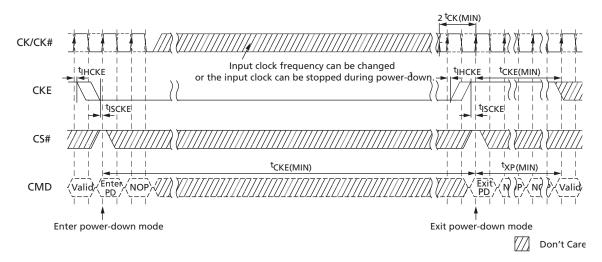
Input clock frequency can be changed or the input clock stopped during power-down, provided that the clock frequency is between the minimum and maximum specified frequencies for the speed grade in use, and that prior to power-down exit, a minimum of two stable clocks complete.
