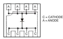
Top View Schematic and Pin Configuration
