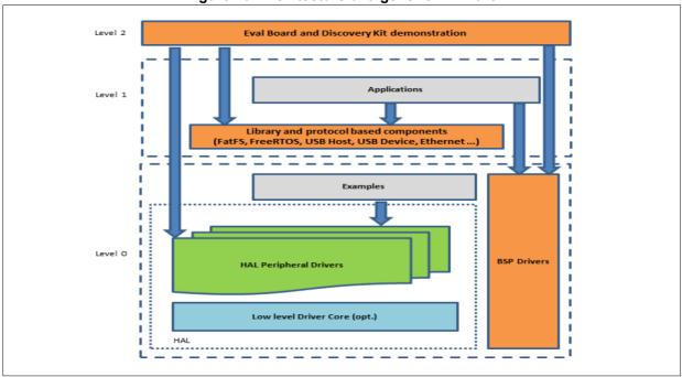
Figure 13. Architecture of a generic firmware
